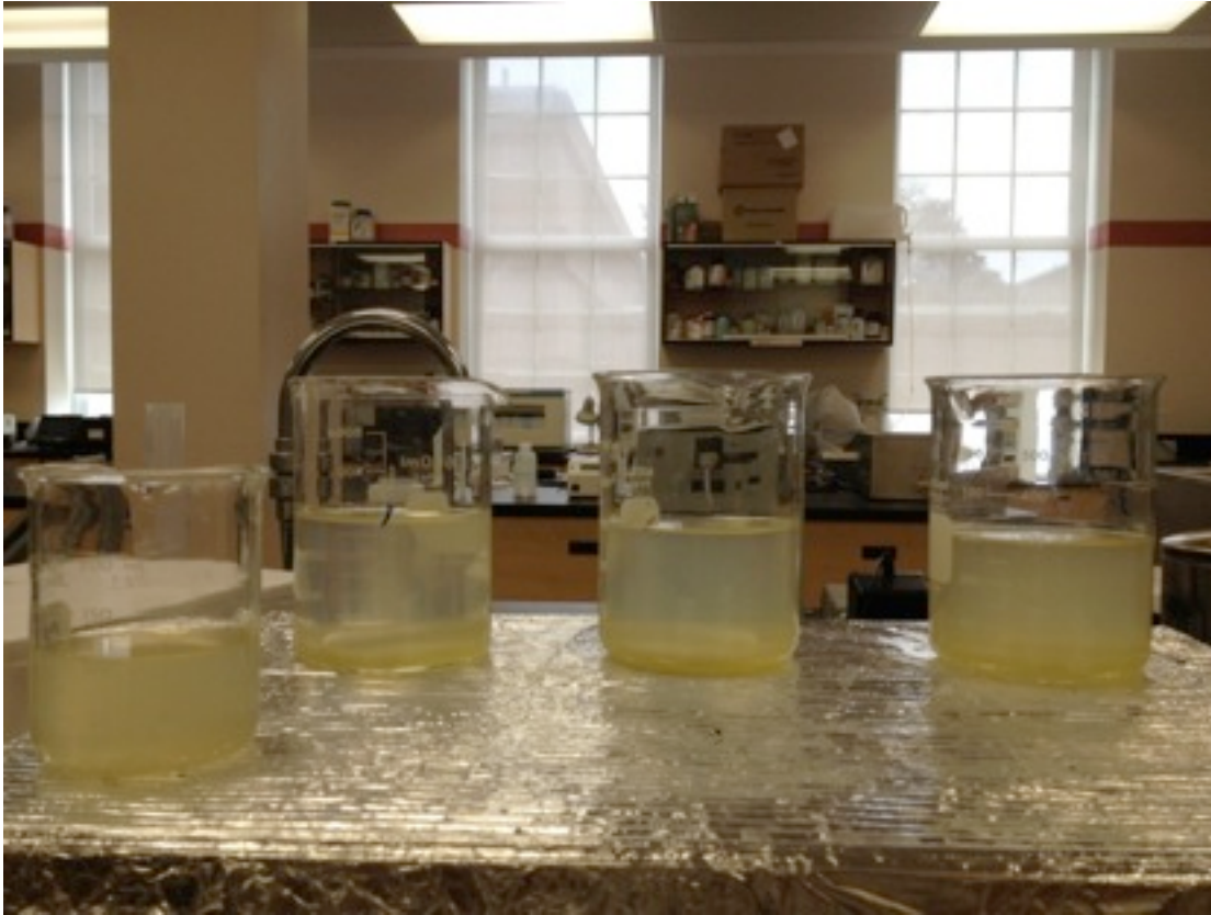
Figure 10: Jar test illustrating the coagulation of organics within lettuce homogenate when treated with sodium aluminate.
