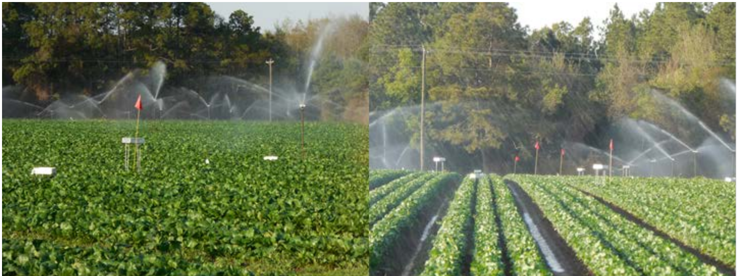
Figure 3. The sampling pans were installed in the study fields prior to an irrigation event and used to capture irrigation water and water splashing from the soil surface. Pans were installed so that pan lips were 2, 4, 8, 16, and 32 inches above the soil surface. Five replicates of each height were installed during each sampling event.
