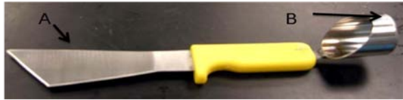
Figure 1. A typical lettuce CIF harvest knife. A. Cutting Blade; B. Coring Ring
