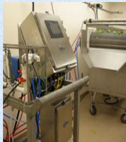
Fig. 1. A pilot plant trial system with T-128 dosing equipment
