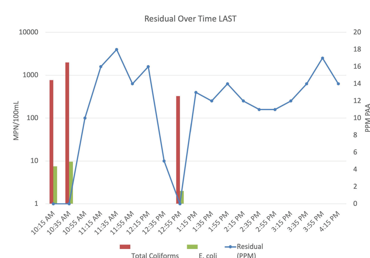
Figure 3. Water Treatment Variability (Last Sprinkler Head)
