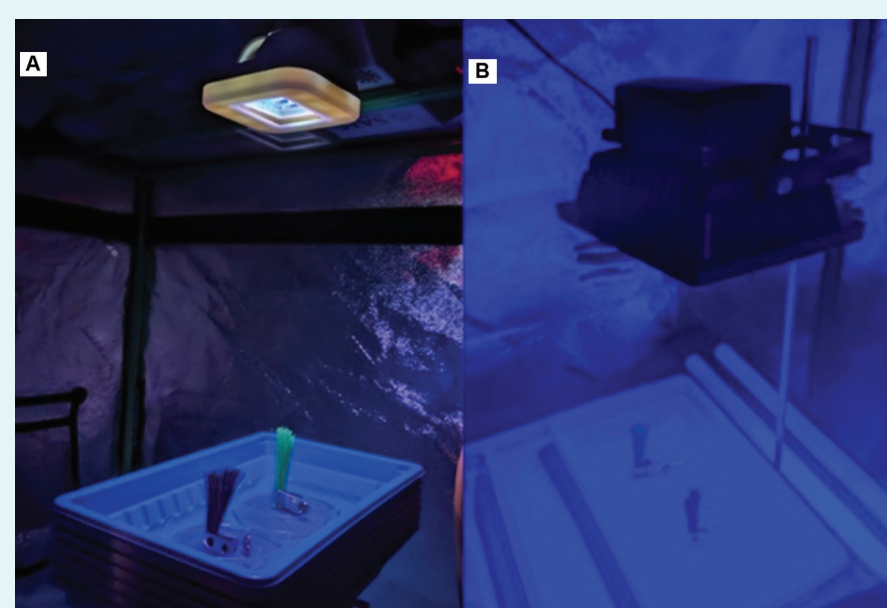
Figure 1: Treatment of brush filaments with antimicrobial lights at 222 nm (A) and 405 nm (B)
