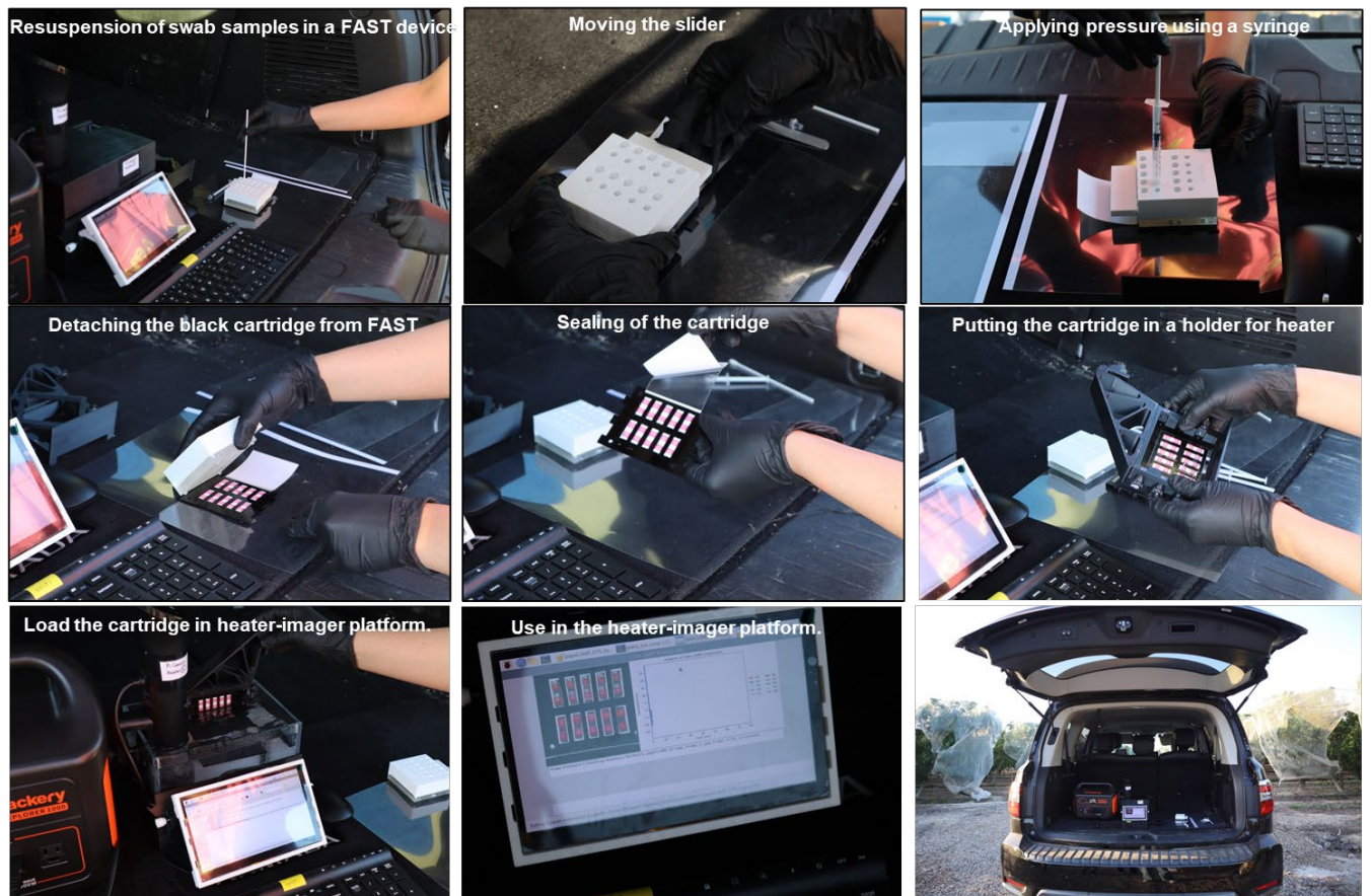
Figure 24: Implementation of Field-Applicable Sampling Tool (FAST) a fully integrated paper-based LAMP testing platform on fresh produce farms in CA (April 2024).
