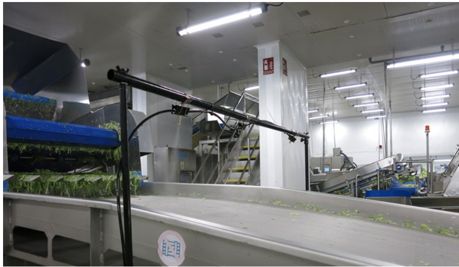
Figure 1. Application device of bacteriophages on the vibration conveyor belt.
