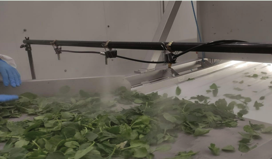
Figure 4. Application of bacteriophages to baby spinach in a commercial processing line
