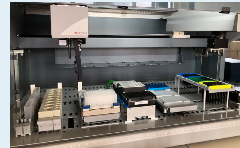
Figure 1. Robotic system housed at the Center for Agricultural Synthetic Biology. The system consists of a TECAN Evo 150 liquid handler and plate mover, 3 Inheco heating/cooling stations, two magnetic bead isolation stations, a plate-based centrifuge, a magnetic stirrer, and an imaging plate reader.
