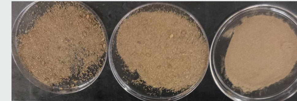
Figure 1. Dust particle sizes used in cross-contamination and transfer studies ( \geq 3,360 \mu\text{m} , >100 \mu\text{m} , <100 \mu\text{m} ).
