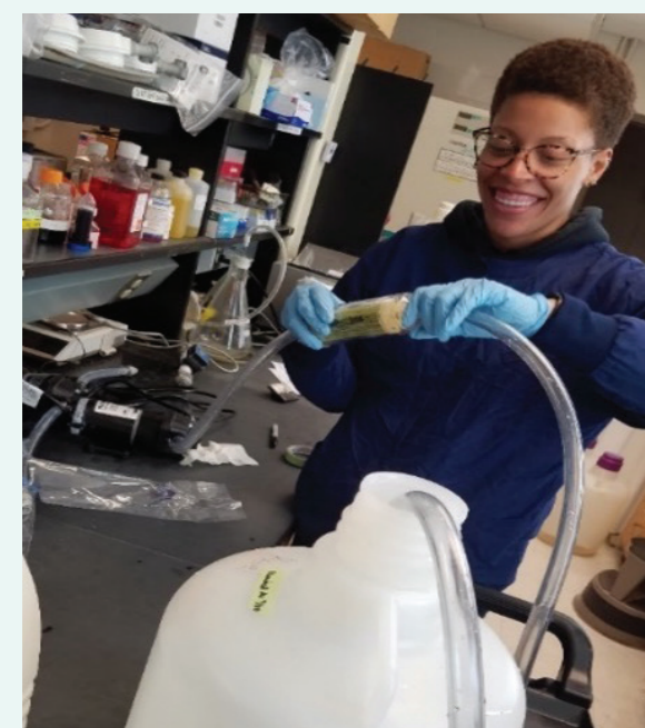
Figure 1. Shani Craighead (graduate research assistant) filtering a water sample collected earlier that day using a modified EPA 1623.1 method.
