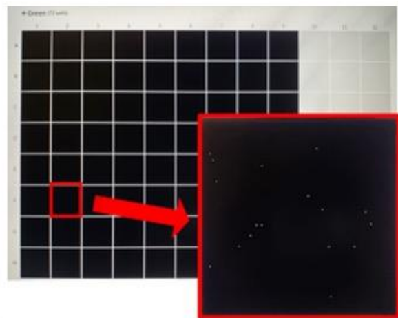
Figure A5. Cyclospora cayetanensis detection visual output in QIAcuity software. Sample P5 in well F2 of the plate is magnified to show the positive partitions in that well.
