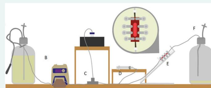
**Figure 1.** Diagram of flow-through biofilm apparatus. Sterile media (A) is pumped through sterile silicone tubing (B-peristaltic pump) to a flow-breaker/air trap (C) and then flow cell which contains the tested surface (E). Microorganisms are inoculated through a separate port (D) with a sterile syringe. Biofilm waste and bulk phase are collected in the waste container (F).
