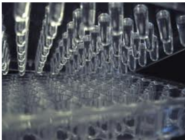
Fig. 1. Image of microtiter plate system for biofilm formation assays. The bottom part is a 96-well microtiter plate; the top part of the image shows the lid with pegs.
