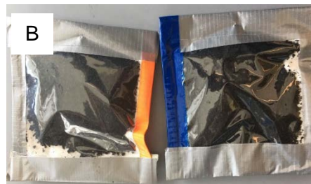
Figure 3B. Customized stainless-steel mesh sampler (A) and color-coded Tyvek pouch containing poultry litter sample (B).
