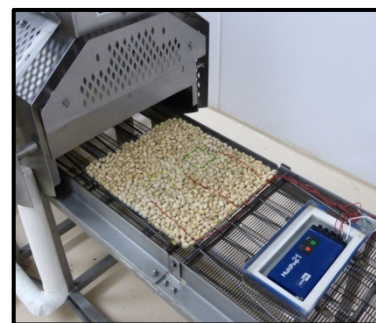
Figure 3. Pilot-scale roasting/pasteurization trials.
