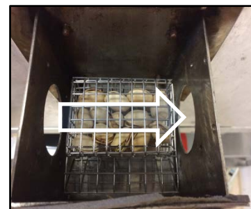
Figure 2. Inoculated pistachios in lab-scale convection oven.
