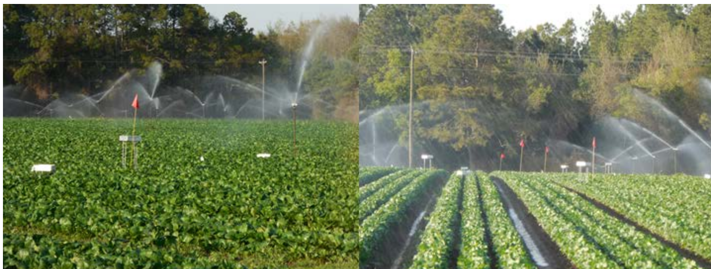
Figure 3. The sampling pans were installed in the study fields prior to an irrigation event and used to capture irrigation water and water splashing from the soil surface. Pans were installed so that pan lips were 2, 4, 8, 16, and 32 inches above the soil surface. Five replicates of each height were installed during each sampling event.
