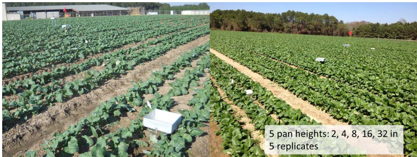
Figure 1. Square aluminum pans were used as samplers for the project. The rim of the pans was installed at five different heights above the soil surface. For each sampling event, there were five replicates of each height.
