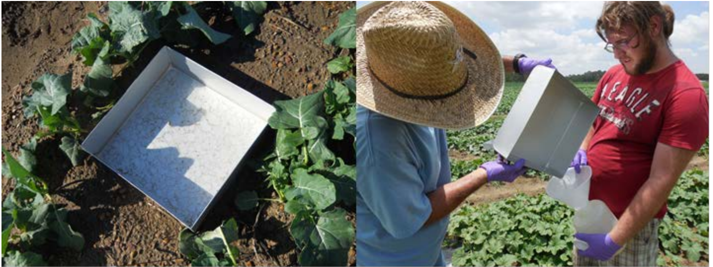
Figure 4. Water and any solids collected in the sampling pans was poured into a sterile sample bottle and returned to the lab for analysis. At the laboratory, the replicates from each height were composited. Only one composite sample was analyzed per height.
