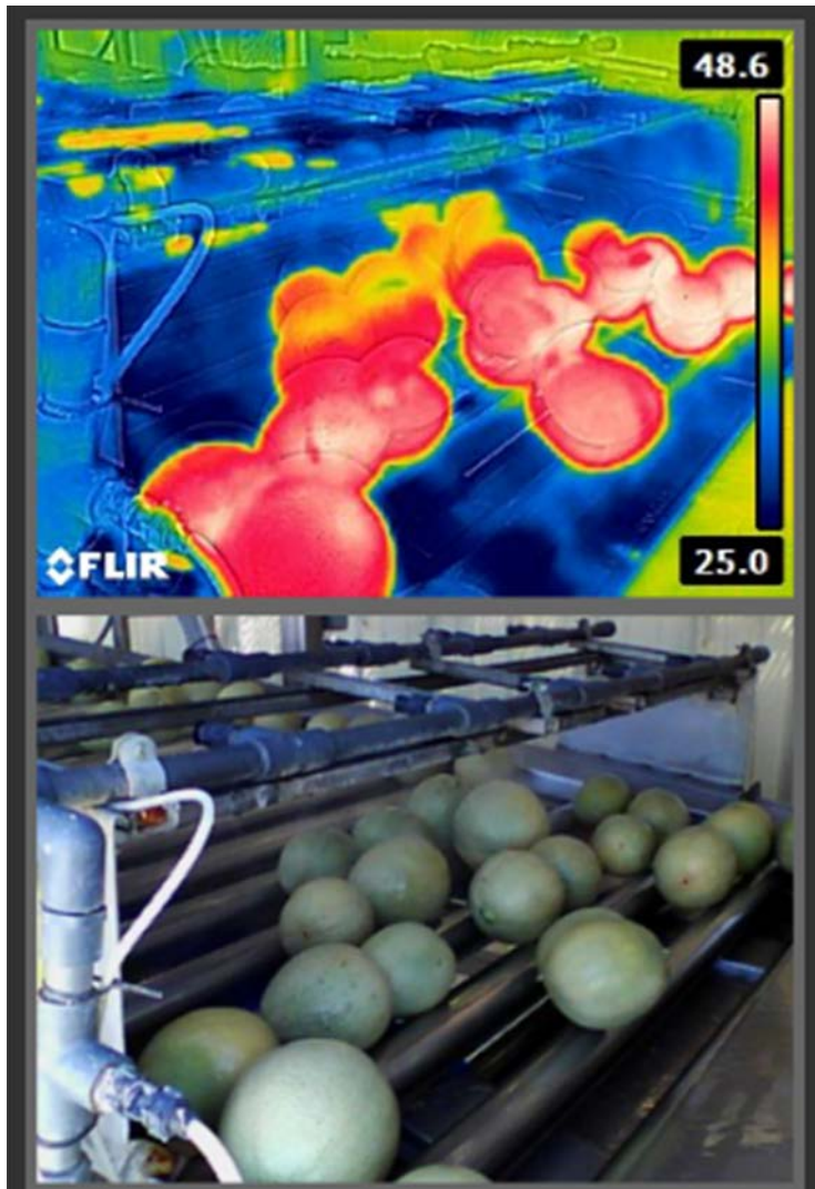
Figure D. Surface Rind Temperatures of whole cantaloupes emerging from the thermal-shower chamber following 15 sec residence at a 60C water temperature.
