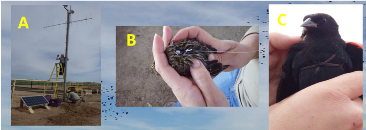
Figure 5. Use of radiotelemetry to track bird movement: (A) solar-powered receiver; (B) bird fitted with a transmitter; (C) "backpack" with transmitter on a red-winged blackbird.
