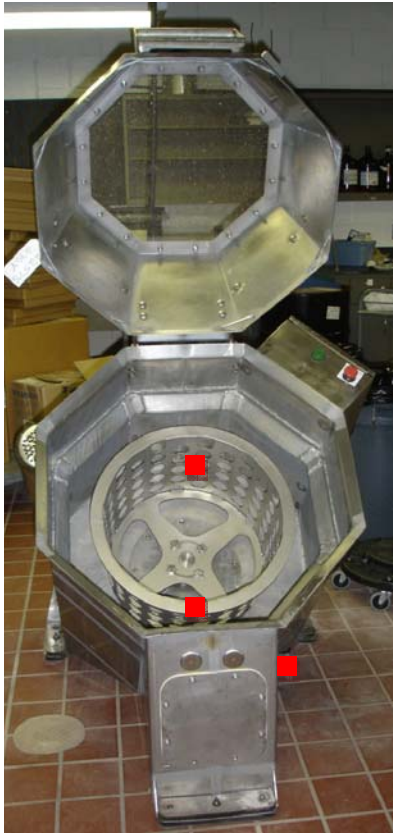
Figure 18. Surface sampling locations (100 cm 2 ) in centrifugal dryer.
