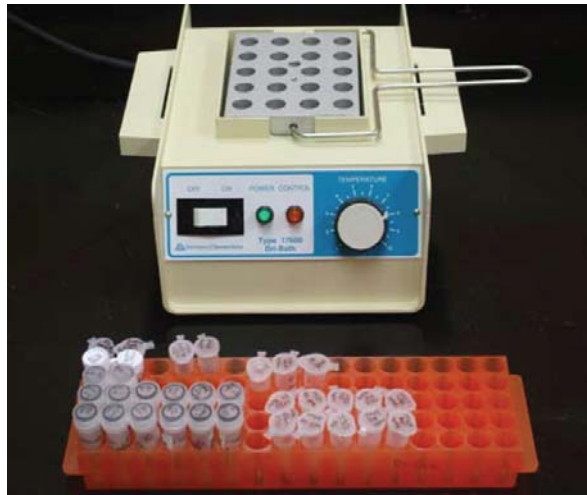
A dry heating block that maintains a constant temperature for performing the LAMP assay.
