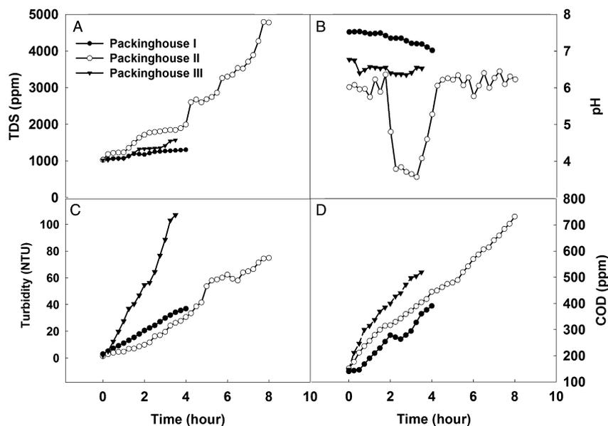
**FIG. 1.** TOMATO DUMP TANK WATER QUALITY PARAMETERS FOR THREE PACKINGHOUSES IN FLORIDA (A) Total dissolved solids (TDS). (B) pH. (C) Turbidity. (D) Chemical oxygen demand (COD).
