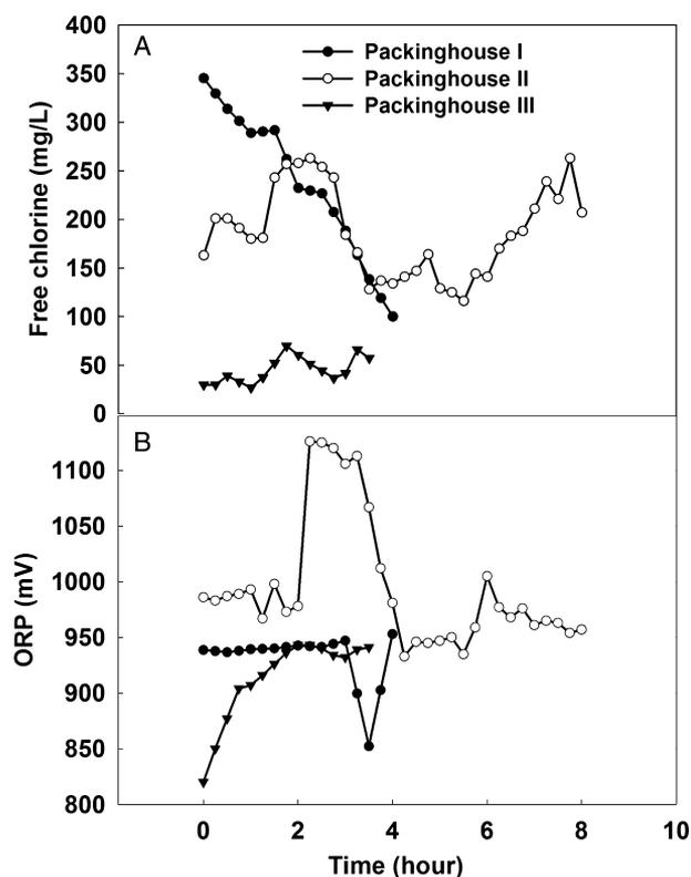
FIG. 2. TOMATO DUMP TANK WATER QUALITY PARAMETERS FOR THREE PACKINGHOUSES IN FLORIDA (A) Free chlorine. (B) ORP.
