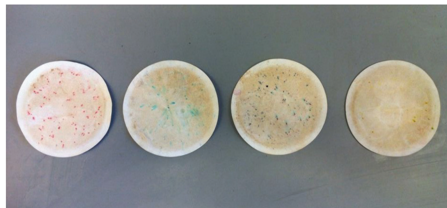
Figure 2. Developed colors on filter papers using color-coded MicroTracers (From left to right: Red, Blue, Violet, Yellow)
