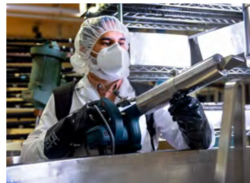
A member of Dr. Snyder's research team demonstrates how superheated steam may be used to hinder pathogens in commercial dry food-processing facilities. Photo: Abby Snyder, Ph.D.
