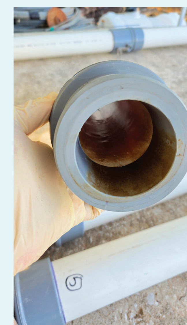
Figure 3: Cross sections of PVC pipe used for mock irrigation of fresh produce with surface water over 28 days showing substantial biofilm development.
