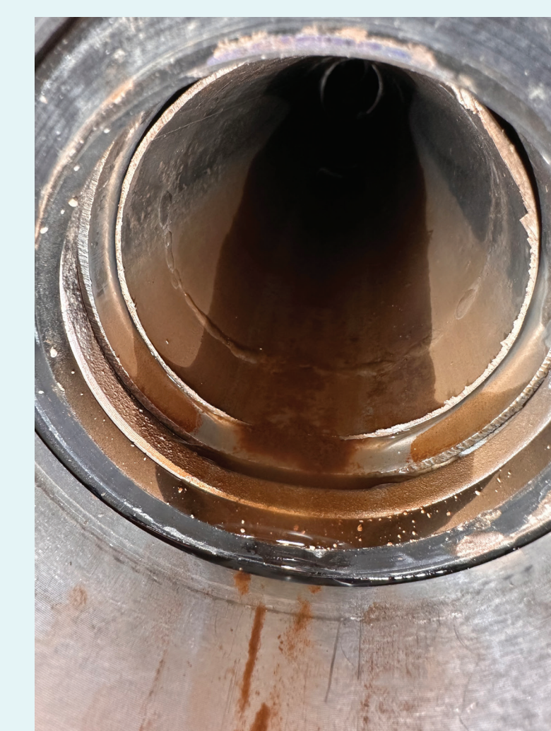
Figure 2: Cross sections of aluminum pipe used for mock irrigation of fresh produce with surface water over 28 days showing substantial biofilm development.
