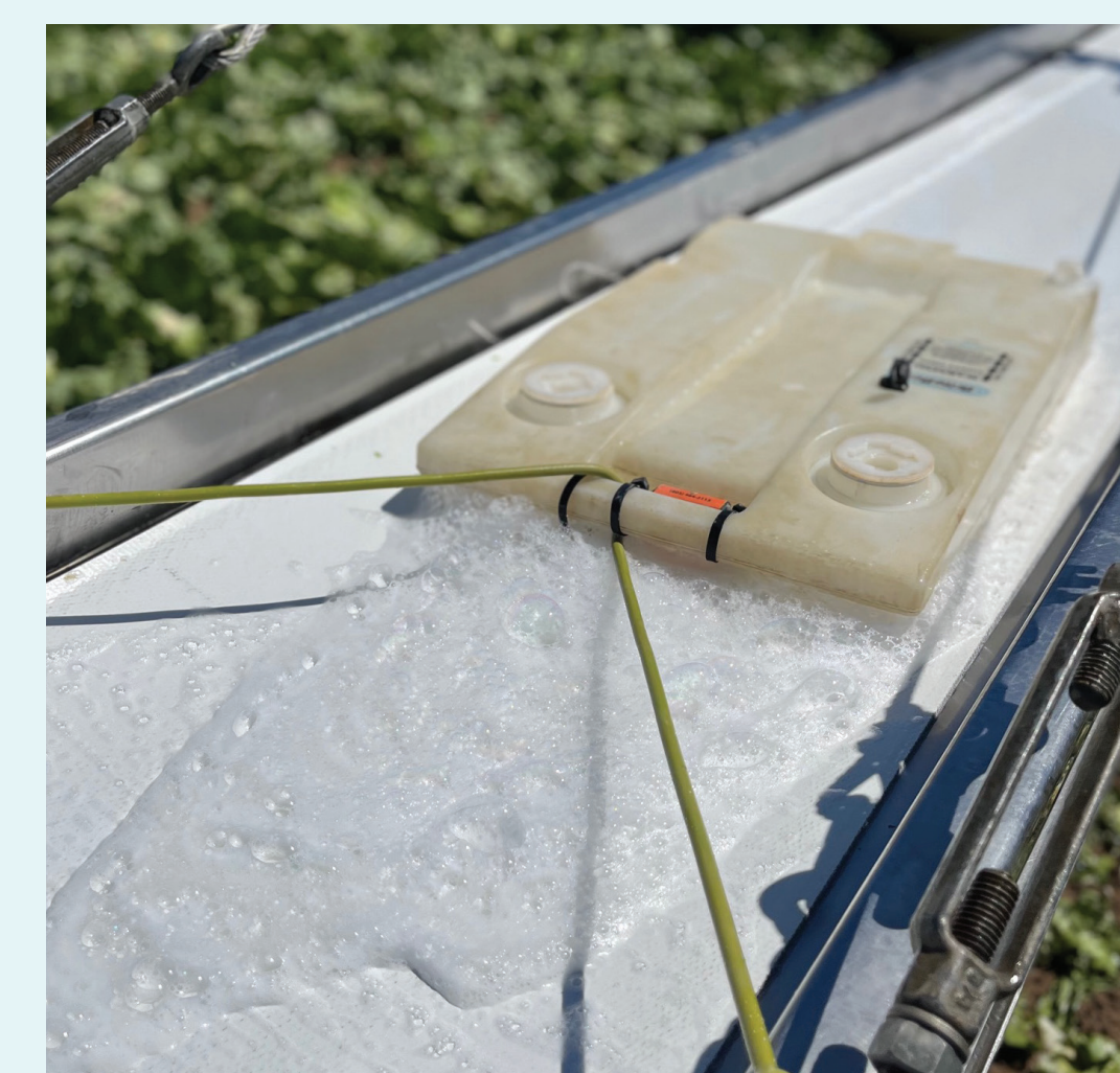
Figure 3: Bright belt to flood detergent or sanitizer on belt surface
